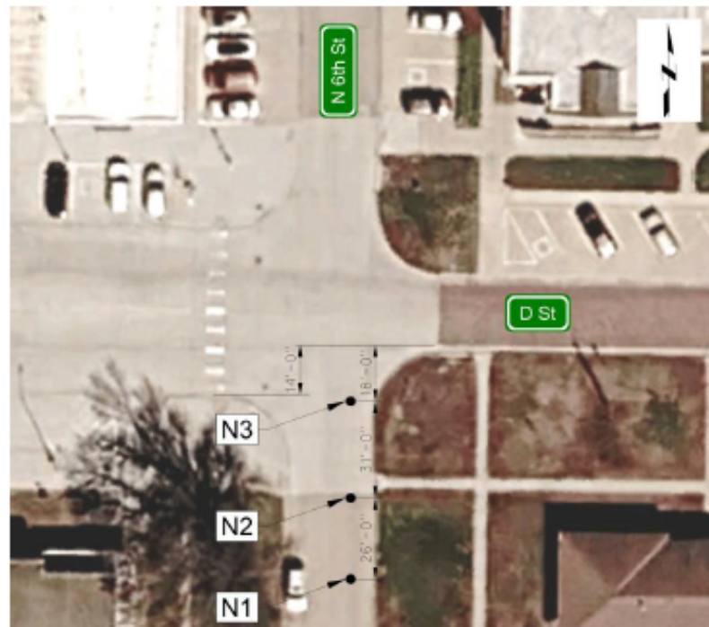
Figure 1: Northbound Sight Distance Measurement Locations
