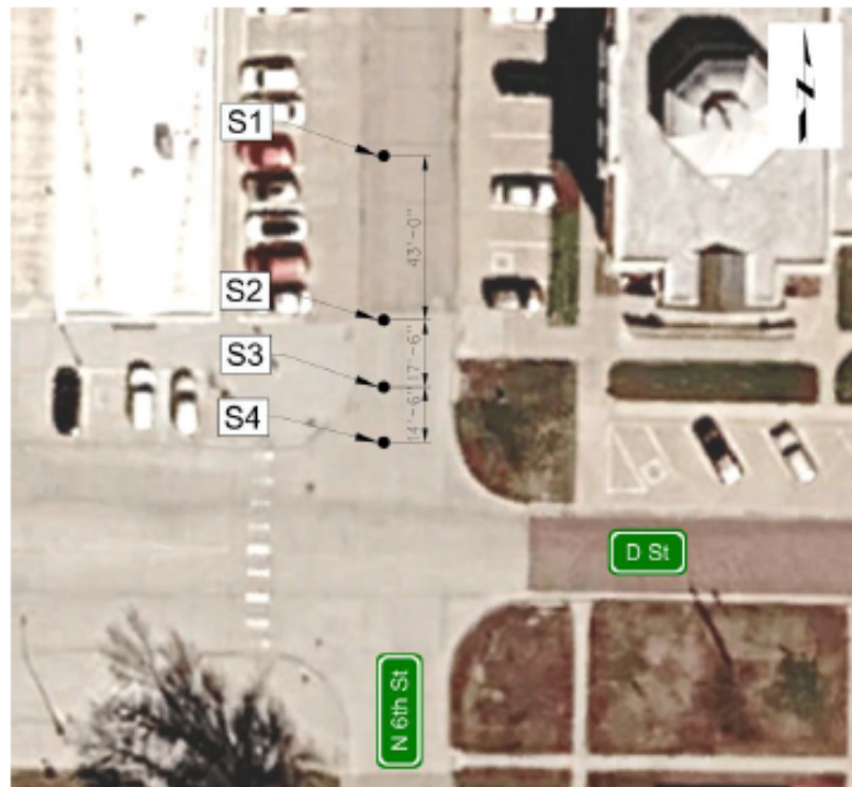
Figure 2: Northbound Sight Distance Measurement Locations
